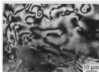
Fig. 8 POM micrograph of solidification-induced band texture in quenched nematic state from 285°C for 4 min to room temperature of a side chain liquid crystalline polymer
